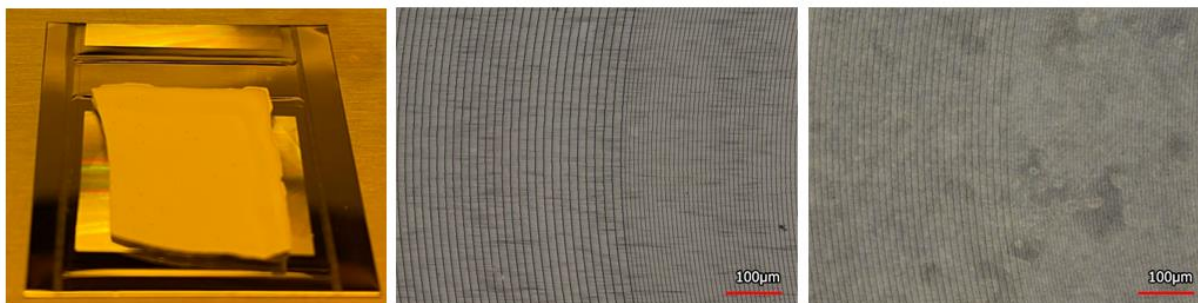
Figure 3. Photograph of green body molding setup on nickel stamp (left) with 0.5 \mu\text{m} 3D surface structures (Fresnel lens) performed at 600 \text{ }^\circ\text{C} . Comparison of replication quality between mold (center) and molded glass (right) with sub- \mu\text{m} roughness.
